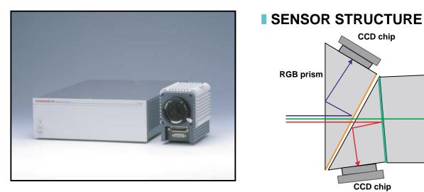
The C7780-10 color camera provides very high fidelity 36 bit real color images in a single exposure, but with independent exposure times for each R,G, and B CCD. Shutter free interline transfer design and cooling of the CCDs to 0°C makes the camera useful for both brightfield color applications as well as high dyanmic range multiple color fluorescence images.
