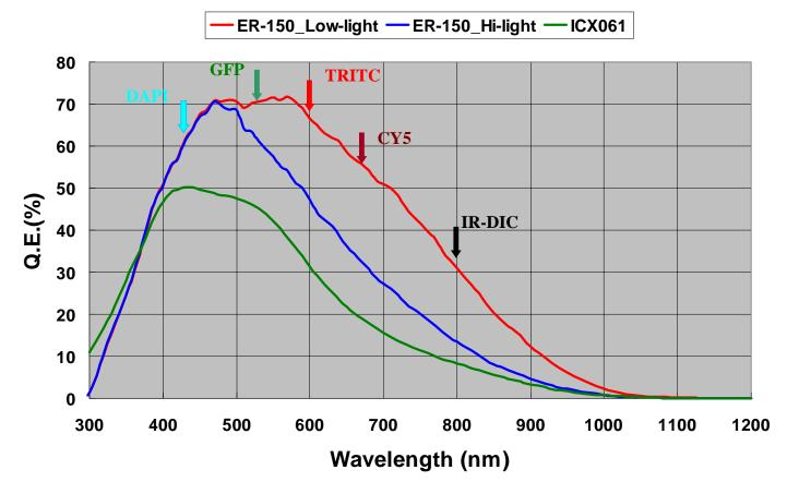
Note: The ORCA ER uses the ER 150 chip The ORCA 100 uses the ICX061 chip
